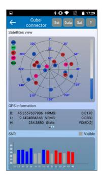
(1) In the figure, the satellite map (GPS visible satellites number + Glonass visible satellites number + BeiDou visible satellites number / the total satellites number)
